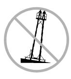
Do not raise the platform unless the machine is level. Do not set the machine up on a surface where it cannot be leveled using only the outriggers.
