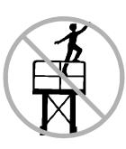
Do not sit, stand or climb on the platform guard rails. Maintain a firm footing on the platform floor at all times.
